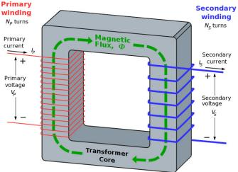
Power (VI) applied to the primary coil is magnetically transferred to the secondary coil, hence the galvanic isolation.
