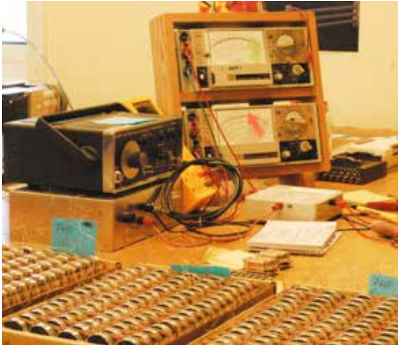
Figure 12: Test station with trays of production units ready for QA (quality assurance) testing.
