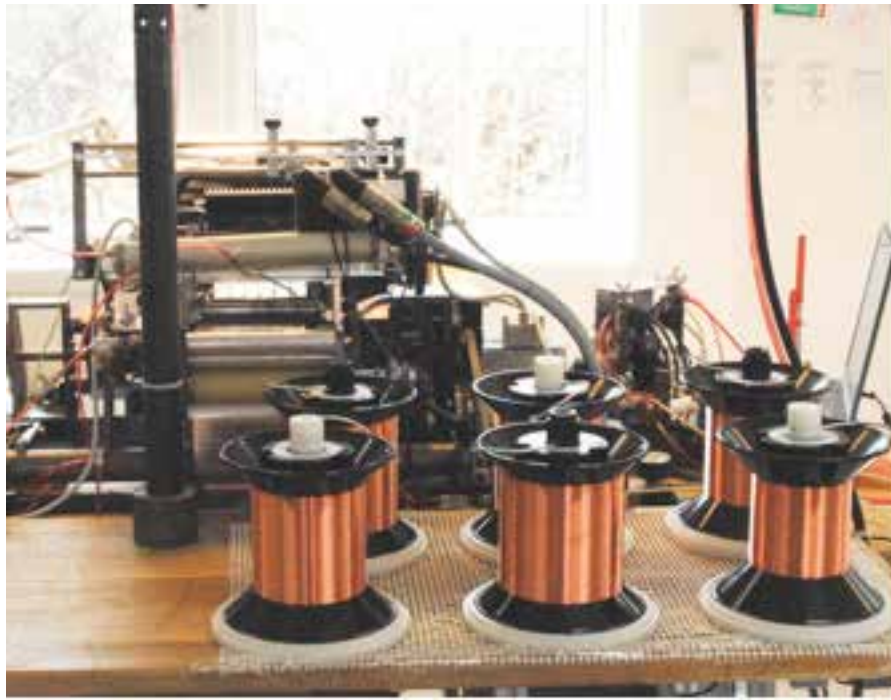
Figure 6: Rear view of a Lundahl coil-winding machine showing wire spools.
