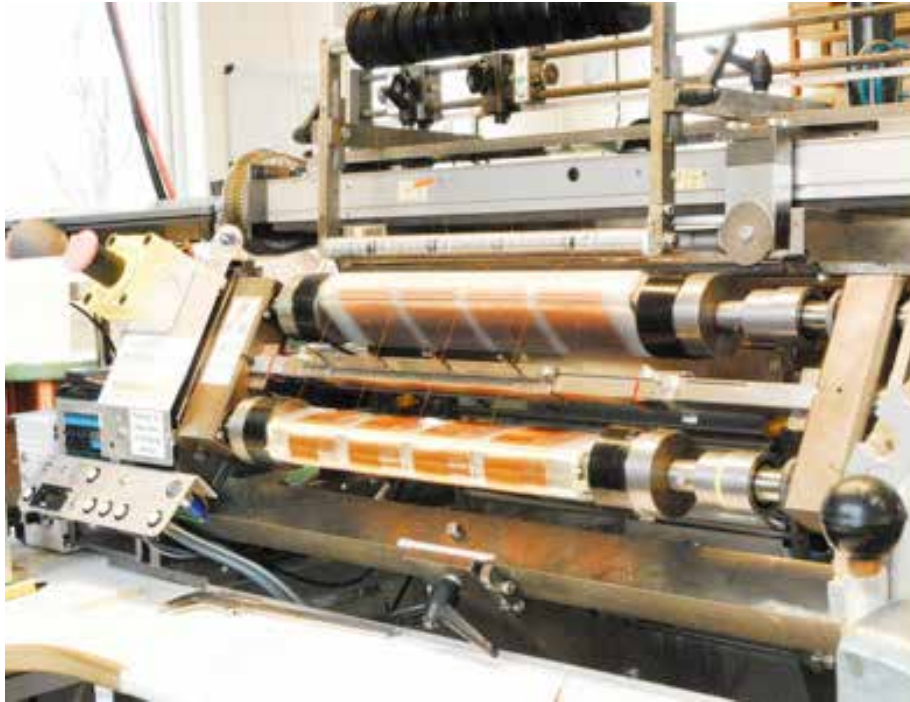
Figure 8: Front view of a Lundahl coil-winding machine for larger format transformers.
