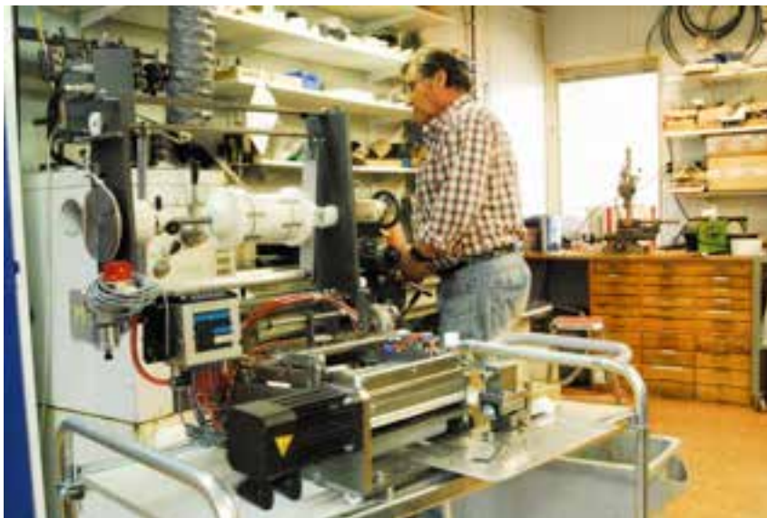
Figure 3: A senior machinist operating a metal lathe with prototype coil-winding machine shown in foreground.
