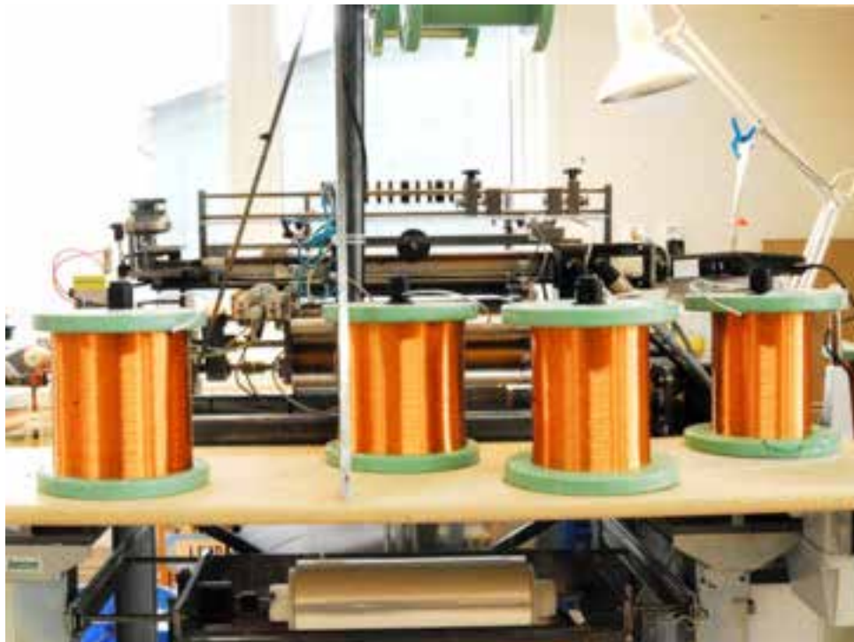
Figure 9: Rear view of large-format Lundahl coil-winding machine showing wire spools.
